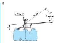
Lever cross-section 1 x 6.4 mm
