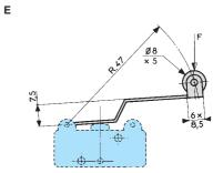
Lever cross-section 1 x 6.4 mm
